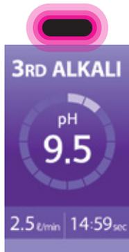
4 When you move your hand close to the proximity sensor the previously selected level (the one with the water droplet on the homescreen) will begin to pour. Move your hand close to the proximity sensor again to stop the flow of water.
